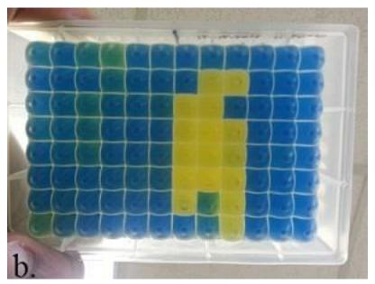
Figure 4.2 Determination of kit specificity with inclusive Vc strains and exclusive non-cholerae Vibrios after incubation at 36 °C for 24 h
