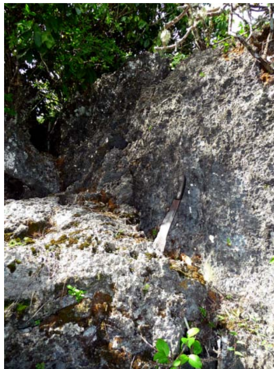
Figure 41 Joint with a possible minor vertical displacement or just a piece of rock fell off on one side of the joint.
