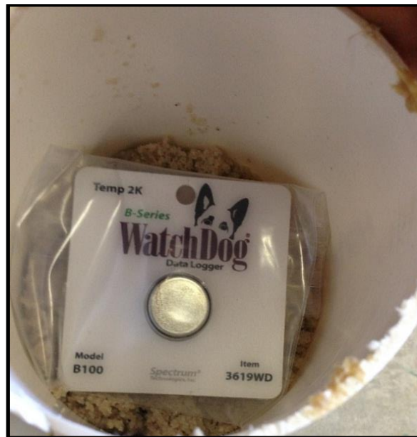
Figure C.10 WatchDog B-Series Button Logger used to record soil temperature of inoculation containers used for pathogenicity evaluations.
