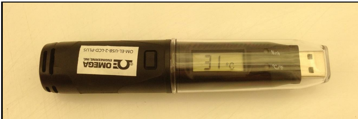
Figure C.12 EL-USB-2-LCD data logger used to measure air temperature, relative humidity, and dew point in growth chambers used for pathogenicity evaluations.
