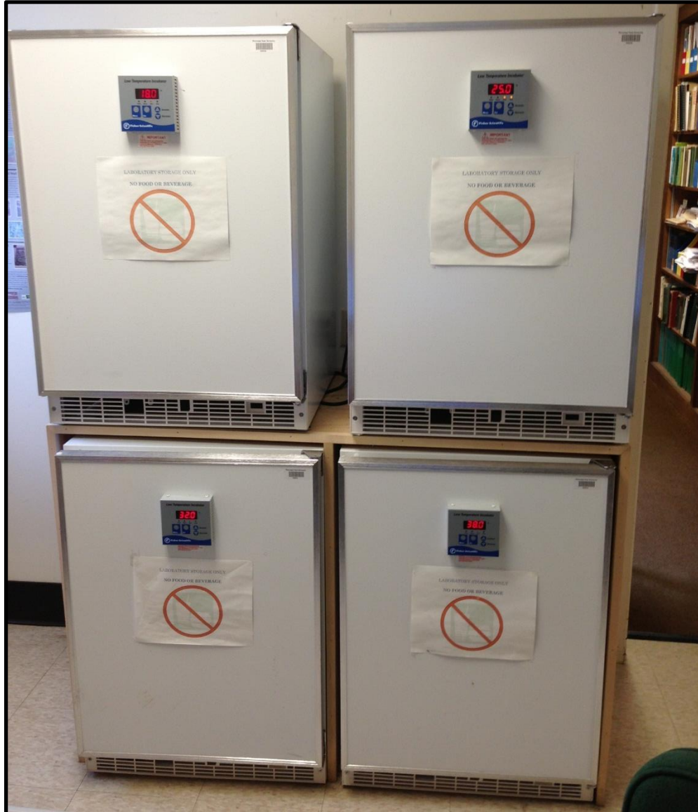
Figure B.15 Incubation chambers set to 18, 25, 32, and 38 C for optimal growing temperature studies of ectotrophic root-infecting fungi.
