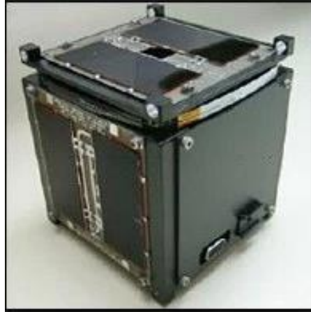
Figure 1.1 Typical 1U Cubesat Structure. [1]
