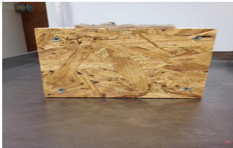
Figure 2.4 The back side of the exterior building wall showing the OSB.
