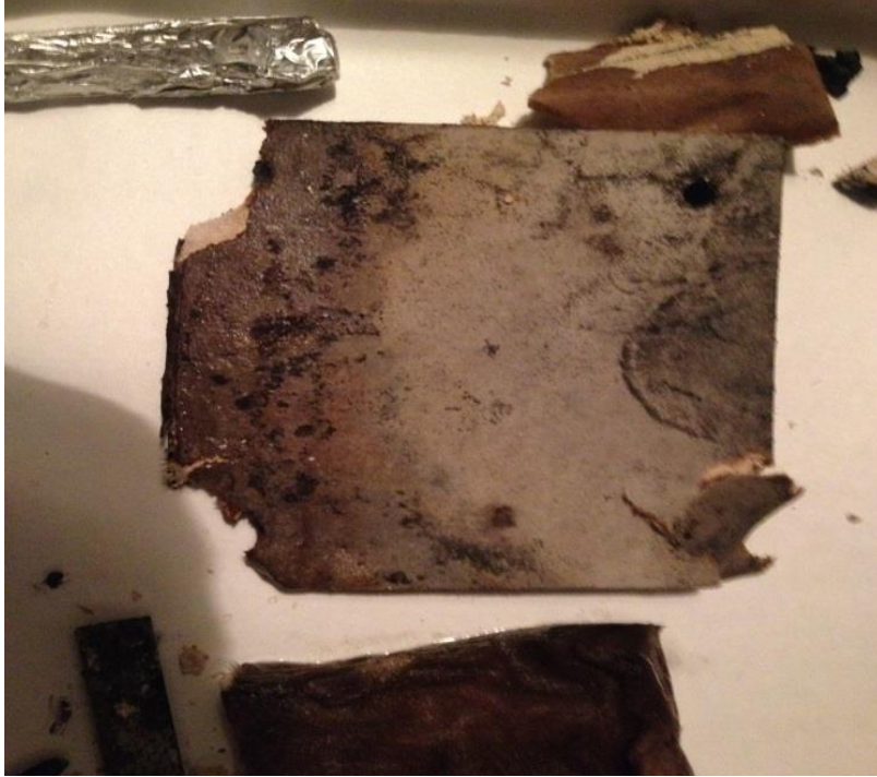
Figure 3.10 Picture of gypsum wallboard surface layer on extraction day 65
