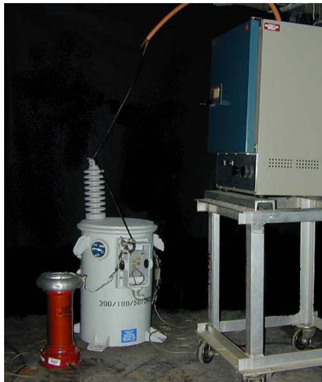
Figure 6.9 Test setup for ac voltage time to breakdown test of NEMA MW 16-C
