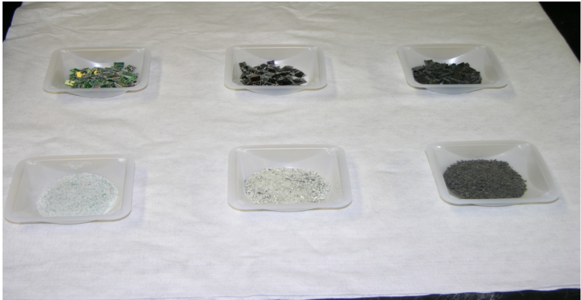
Figure 2.9 Composite of PWB, LCD screen and Casing Samples Used In Experiments
