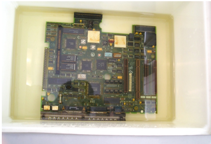
Figure 2.17 Top View of Dynamic Leach Apparatus with a PWB
