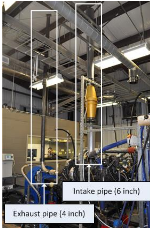
Figure 6.6 Intake and exhaust plumbing with vertical orientation
