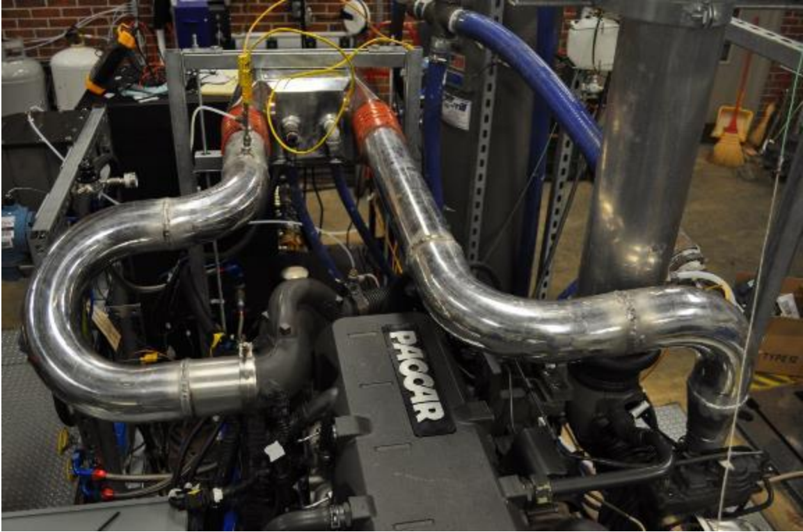
Figure 6.8 Intake charge air plumbing
