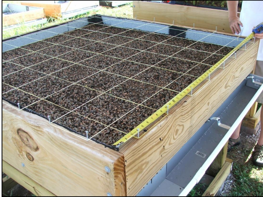
Figure 3.2 All green roof platforms were equipped with a grid point frame indicating the planting locations.
