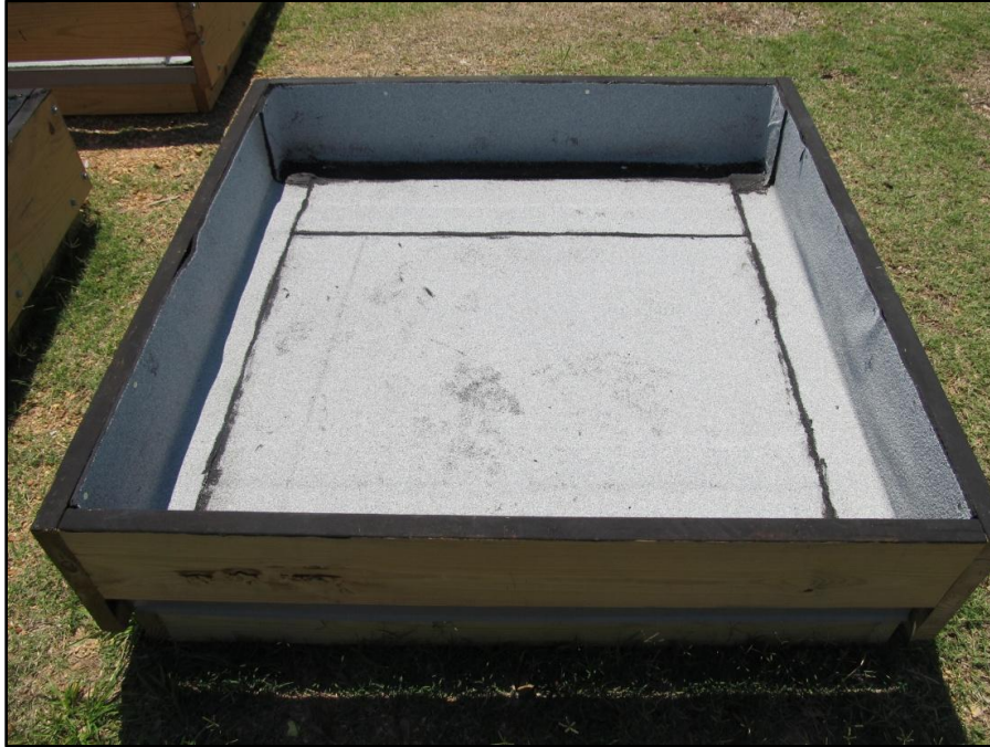
Figure 3.1 Wood-frame platforms constructed with treated pine lumber having 4' × 4' internal dimensions and 8" side walls. All green roof platforms were equipped with waterproofing membrane, moisture retention mat and platforms with 33% slope were equipped with a soil stabilizer layer.
