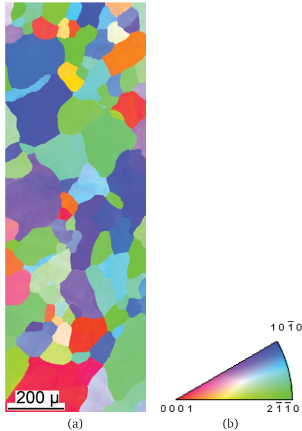
Figure 3.2 EBSD texture analysis of initial state of pure Magnesium.
