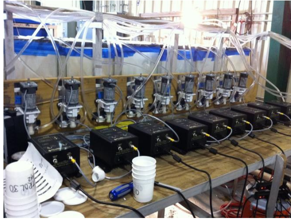
Figure 3.9 Variable flow rate pumps (QV300, Fluid Metering, Inc., Syosset, NY)
