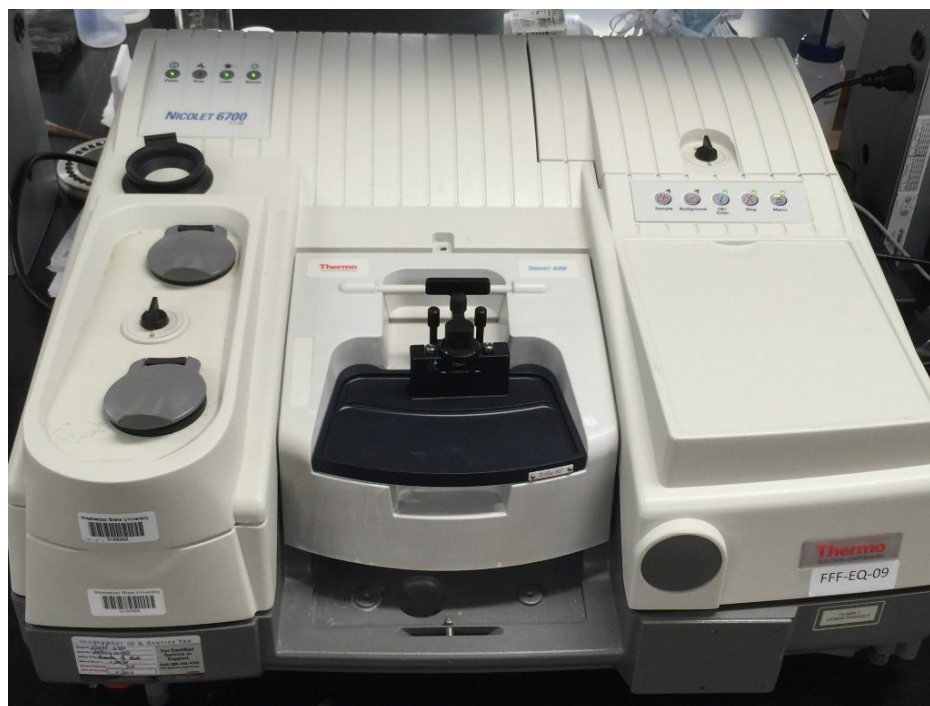
Figure 2.2 Thermo Nicolet 6700 FTIR optical spectrometer equipped with a liquid nitrogen-cooled MCT High-D detector, KBr beamsplitter, and Smart ARK accessory with a ZnSe horizontal attenuated total reflectance crystal at a 60° angle of incidence.
