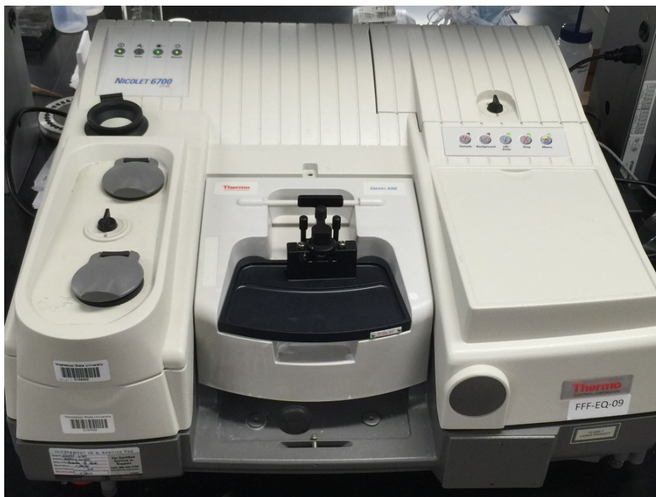
Figure 3.2 Thermo Nicolet 6700 FTIR optical spectrometer equipped with a liquid nitrogen-cooled MCT High-D detector, KBr beamsplitter, and Smart ARK accessory with a ZnSe horizontal attenuated total reflectance crystal at a 60° angle of incidence.
