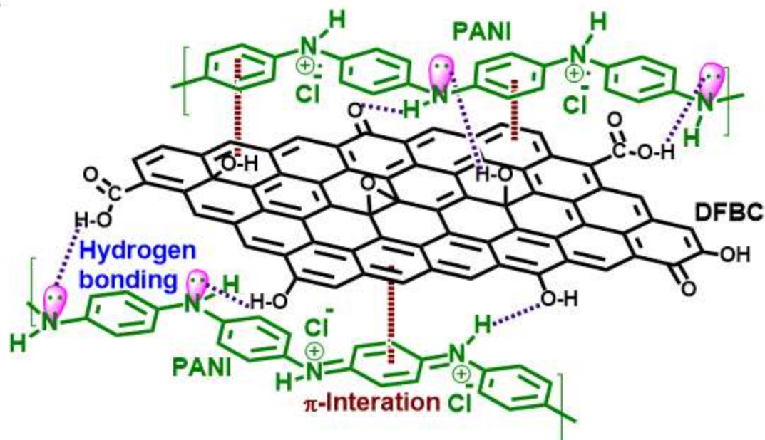
Figure 3.7 Illustration of the interaction between PANI and biochar at their interface
