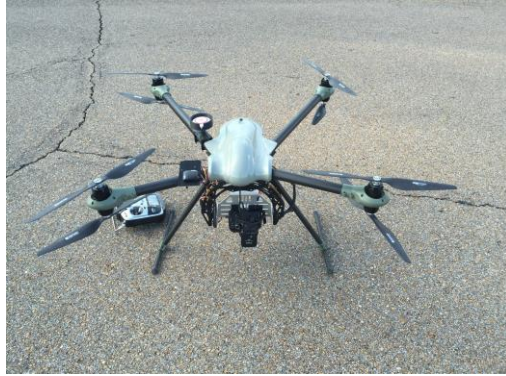
Figure 4.1 Drone used in testing for taking aerial photographs of the tractor-dolly system
