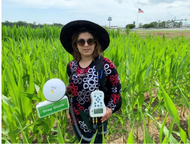
Figure 4.2 Crop Circle ACS-430 and GeoSCOUT X datalogger connected to RTK GPS.
