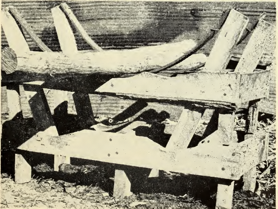
Figure 5. Post-bundling rack. The two bowed irons on which the posts are laid conform to the curve of the bottom of the treating tanks.
