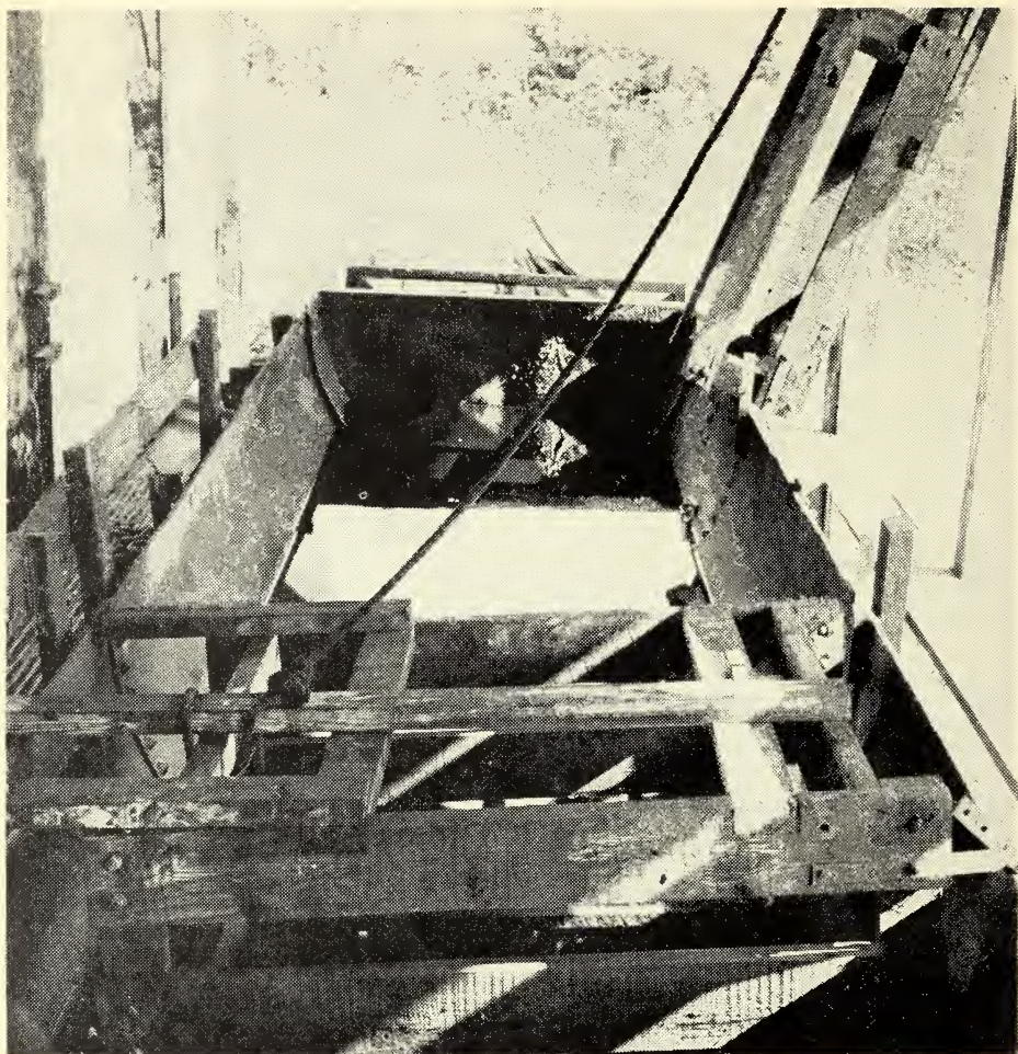
Figure 6. Heavy wooden frames, hinged to the sides of the tanks, are dropped on the bundles of posts to keep them submerged in the preservative.
