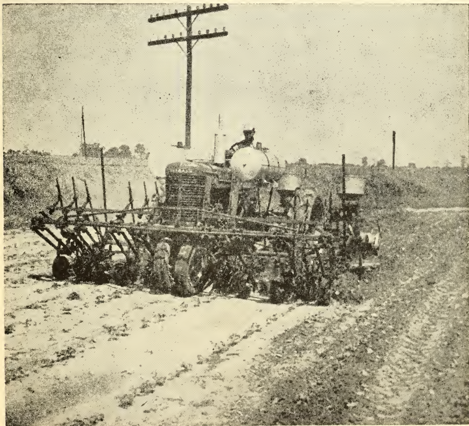
Figure 3. Cultivating young cotton plants with a front-mounted cultivator equipped with rotary hoe attachments. The rear-mounted planter may be used for late planting or for planting skips in the field without changes in the equipment.
