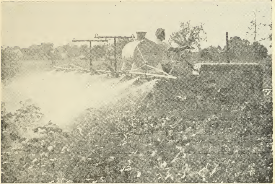
Figure 8. Applying a liquid defoliant with an eight-row tractor-mounted sprayer. Wide booms and tractor shields are essential to reduce plant damage by the machine.
