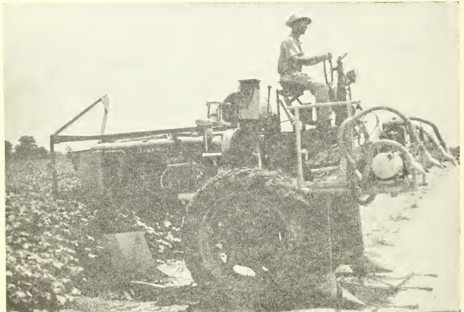
Figure 7. A cotton picker tractor equipped with a duster and wheel shields for the application of insecticides in rank cotton.
