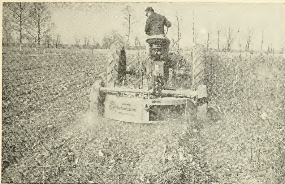
Figure 1. A power-driven horizontal blade type stalk shredder operating in rank cotton stalks.
