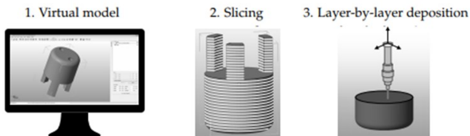
Figure 6.1 Steps of 3D printing [45].
