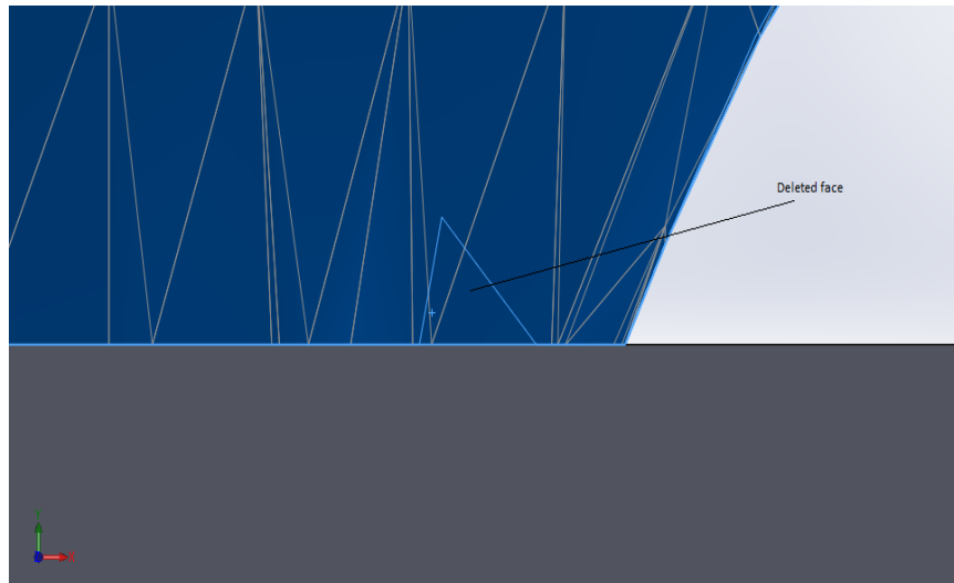
Figure 4.8 Example of a surface gap.
