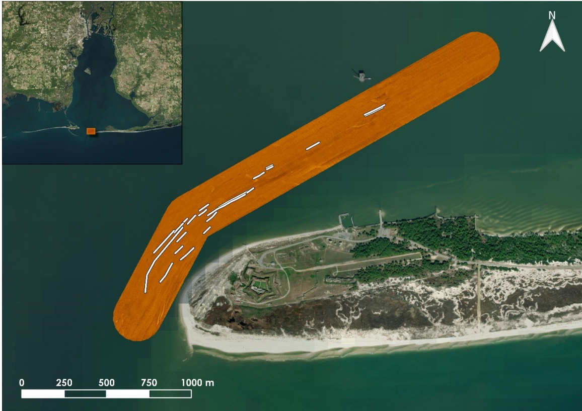
Figure 1.4 Image of the sea floor captured during the side-scan sonar survey of the Channel, including trawl scars marked with white lines.
