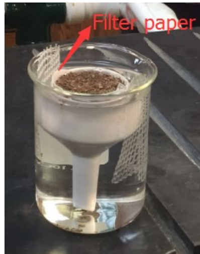
Figure 2.10 Soil substrate filled in a Buchner funnel in a beaker
