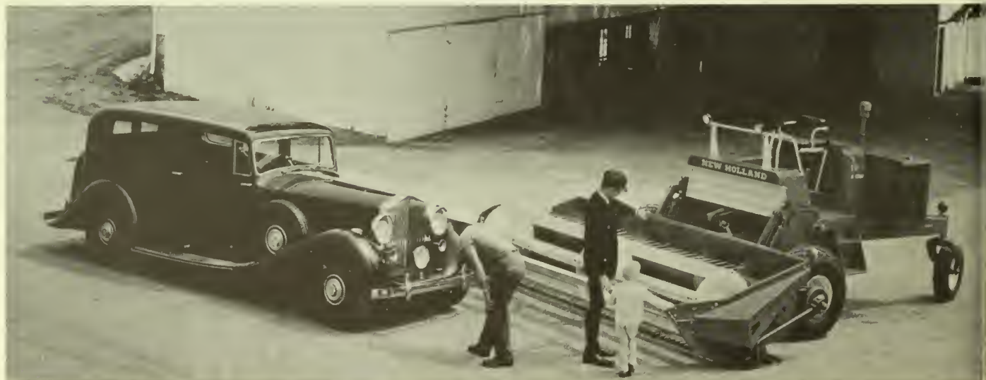
Figure 2. A self-propelled harvesting machine (right) for cutting, conditioning and wind-rowing alfalfa.
