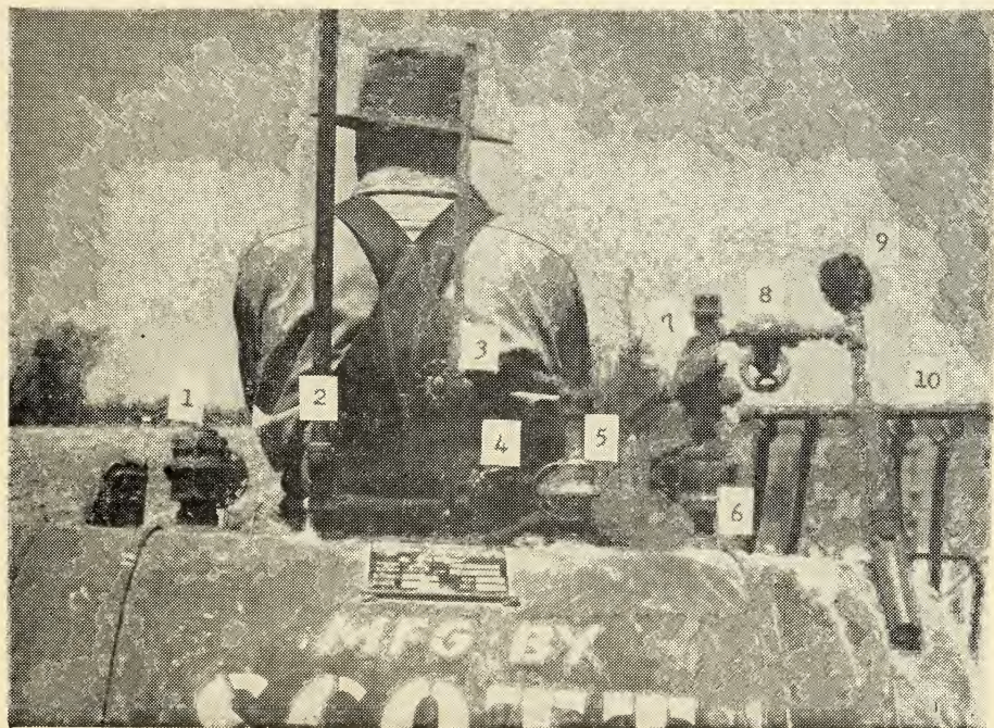
Figure 9. Fittings for anhydrous ammonia tractor tank. (1) Vapor line return valve for filling with pump or compressor. (2) Pop-off valve with stand pipe. (3) Bleed-off and stationary fill gauge valve and stand pipe. (4) Tank pressure gauge. (5) Filling valve. (6) Feed line valve. (7) Quick cut-off valve. (8) Regulating needle valve. (9) Low pressure gauge. (10) Manifold.
