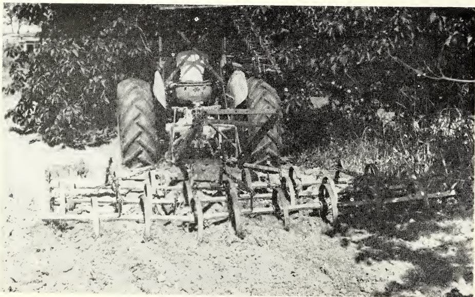
Figure 9. A spring-tooth harrow will maintain a weed-free orchard during the summer if spring cultivation has been thorough. This implement is less destructive to tung feeding roots than is a disk.
