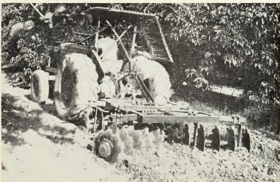
Figure 7. A wide tandem disk can be used to turn under old leaves and weeds in the middles.
