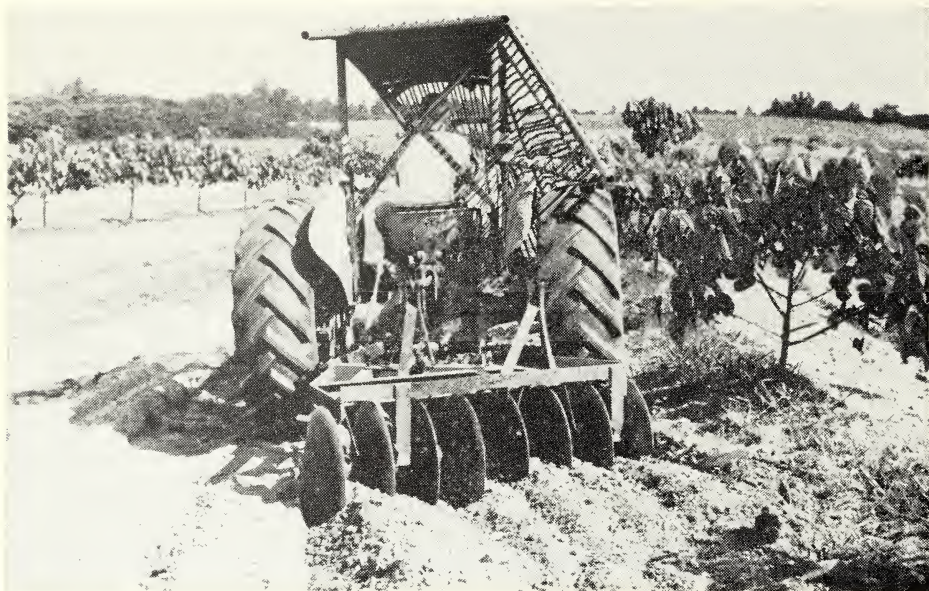
Figure 4. A one-way disk should be used to build terraces along the contoured tree rows in young orchards. By adjusting its pitch, this implement can be used to maintain these terraces after they have been formed.
