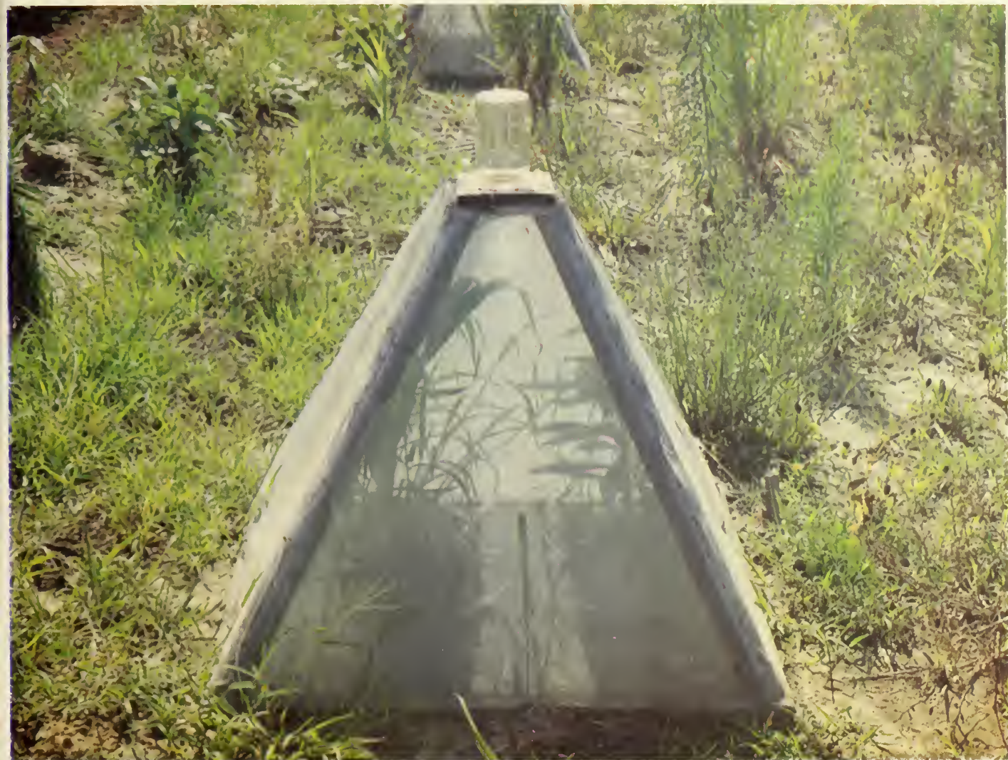
Figure 3. Pyramid-shaped cage 1 yard square at the base, covered with a fine mesh nylon screen and fitted with a quart jar on top.
