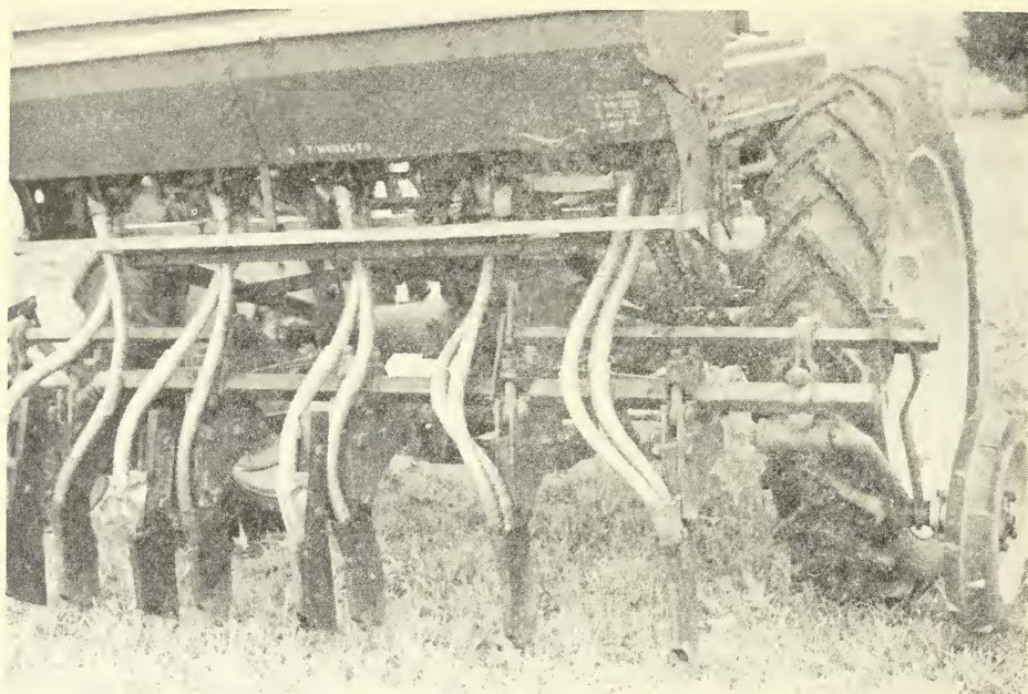
Figure 1. Experimental equipment developed to study the principles of seeding and fertilizing supplementary winter growing crops in a permanent pasture sod. Note arrangement for obtaining fertilizer placement variable.
