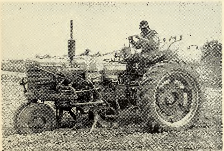
This tractor is equipped to apply anhydrous ammonia, a mixture of superphosphate and potash, and plant seed in one operation.
