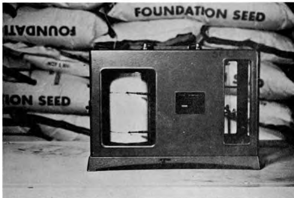
Figure 3. Foundation seed stored under low temperature, low relative humidity conditions. Hygrothermograph records the temperature and relative humidity of the air.
