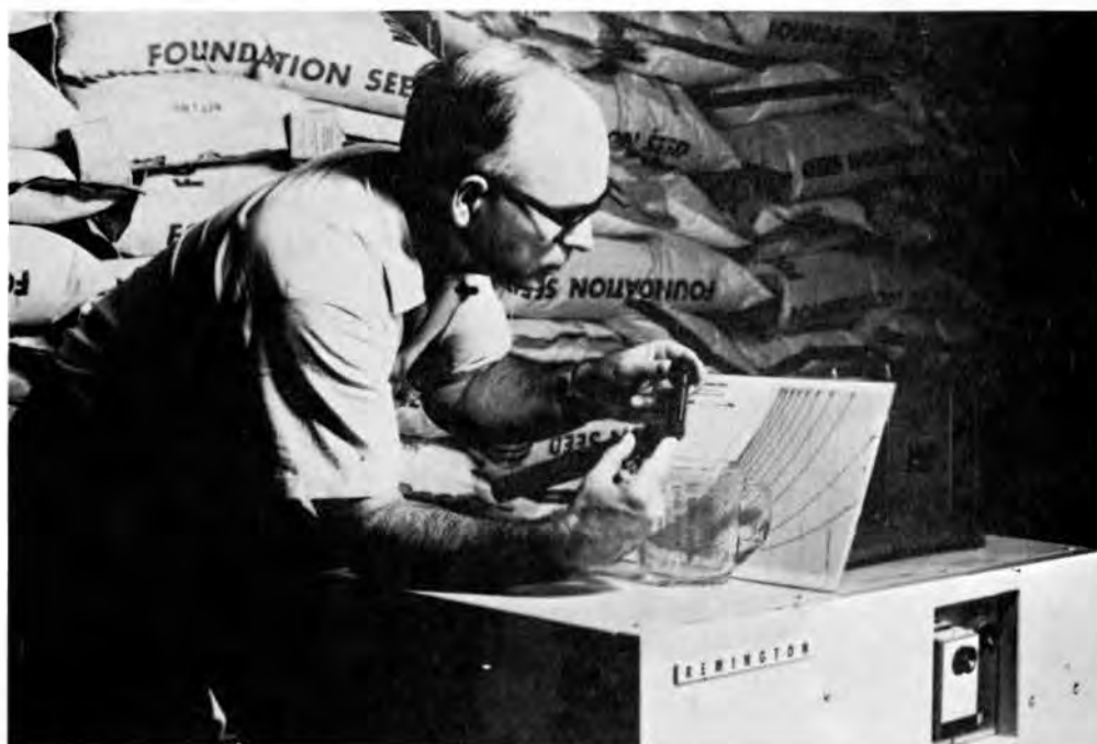
Figure 4. A sling and psychrometric chart is used to determine the properties of air inside a seed storage room.
