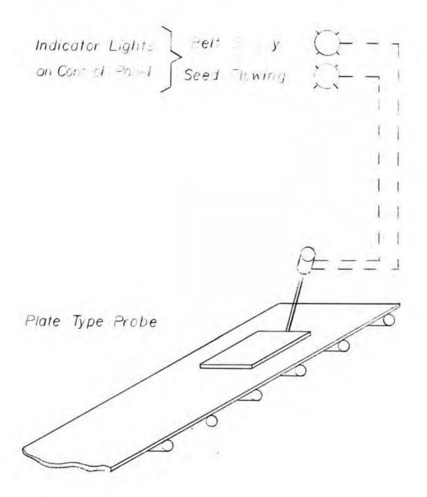
Drawing No. 3 shows how a level switch can be used to determine when a conveyor belt is empty or full. This unit assists the operator by preventing mixing of seed and by getting maximum use out of a conveying system. A flat plate type probe is used for this application.
