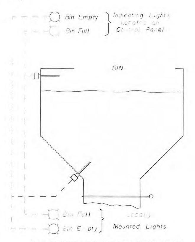
Drawing No. 1 shows how you can use two on-off type probes for indication of the level of seed in a bin. These units can be used for indication only or they can be tied into an automatic plant system and be used to stop and start conveyors, as safety shutdowns, etc.
