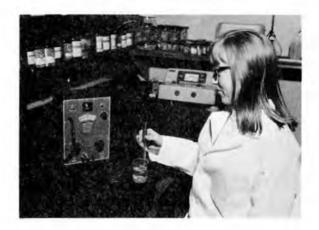
Figure 4. Measurement of electrical conductivity.
