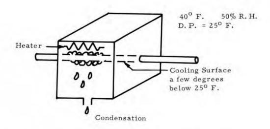
Figure 2. To maintain a particular temperature and relative humidity, the temperature of the cooling coil must be a few degrees below the dewpoint temperature. 59
