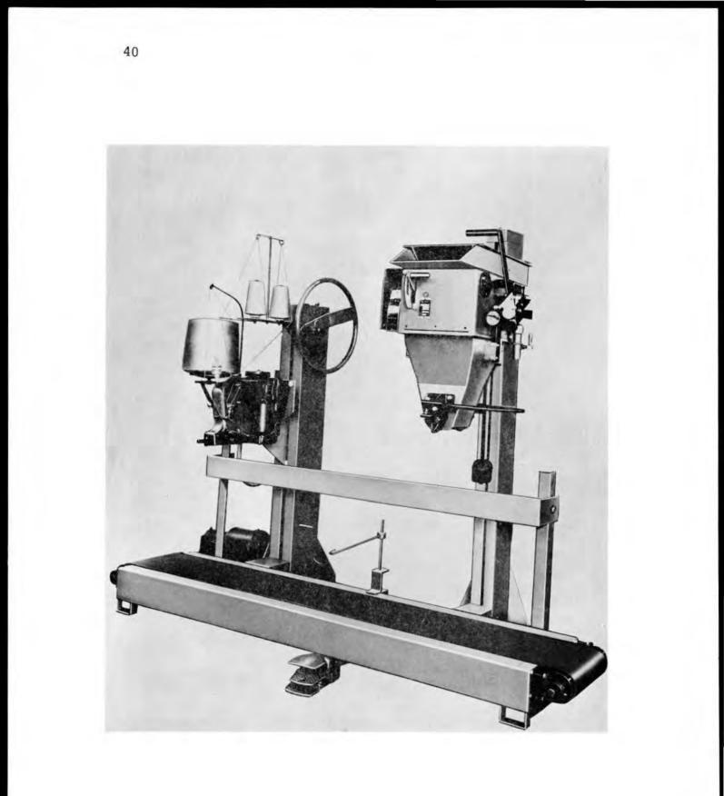
Figure 1. Equipment for a one-man bagging operation.
