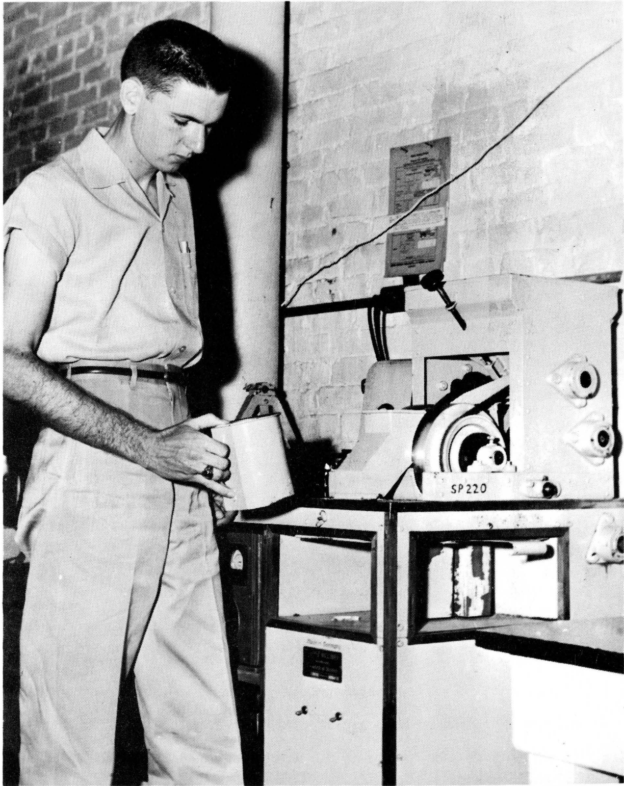
Gompper Laboratory Magnetic Cleaner used in the Seed Technology Laboratory for research and for assisting seedsmen with separation problems.
