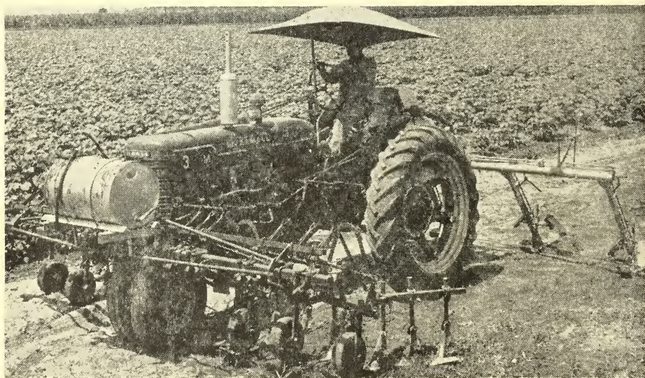
Figure 7. The use of flame cultivation equipment in combination with a standard cultivator reduces the cost of operation.
