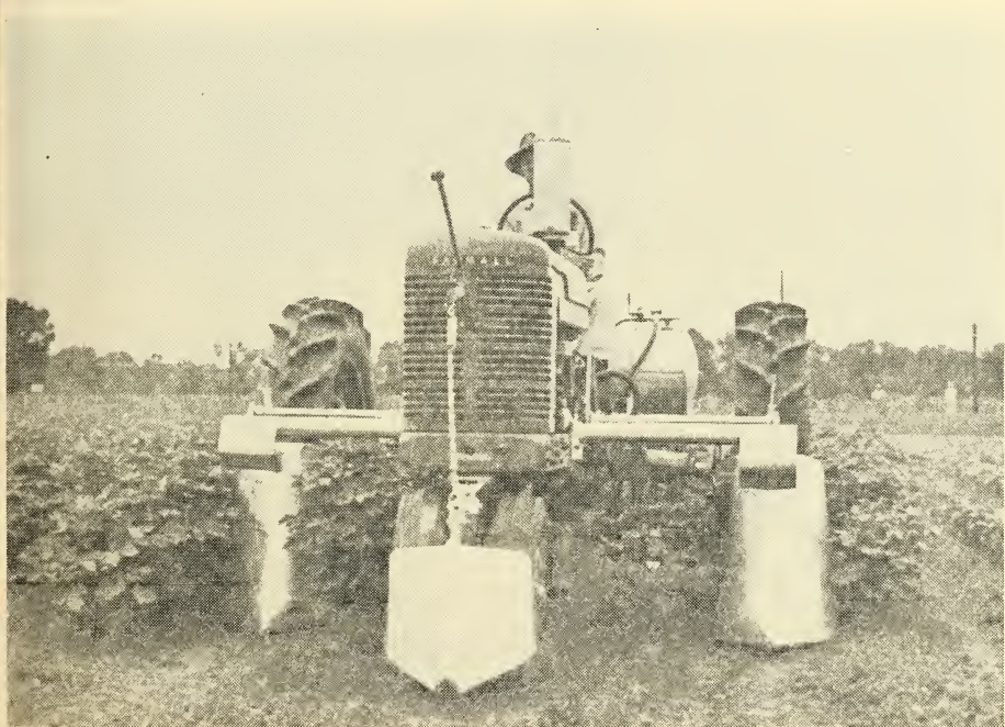
Figure 9. Tractor wheel shields reduce stalk damage when farming late-season or rank cotton.
