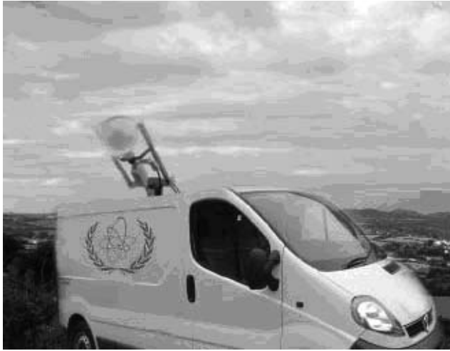
Figure 10. A mobile on-site laboratory samples and concentrates atmospheric-borne pollutants. Local meteorological conditions and the GPS location are also recorded.
