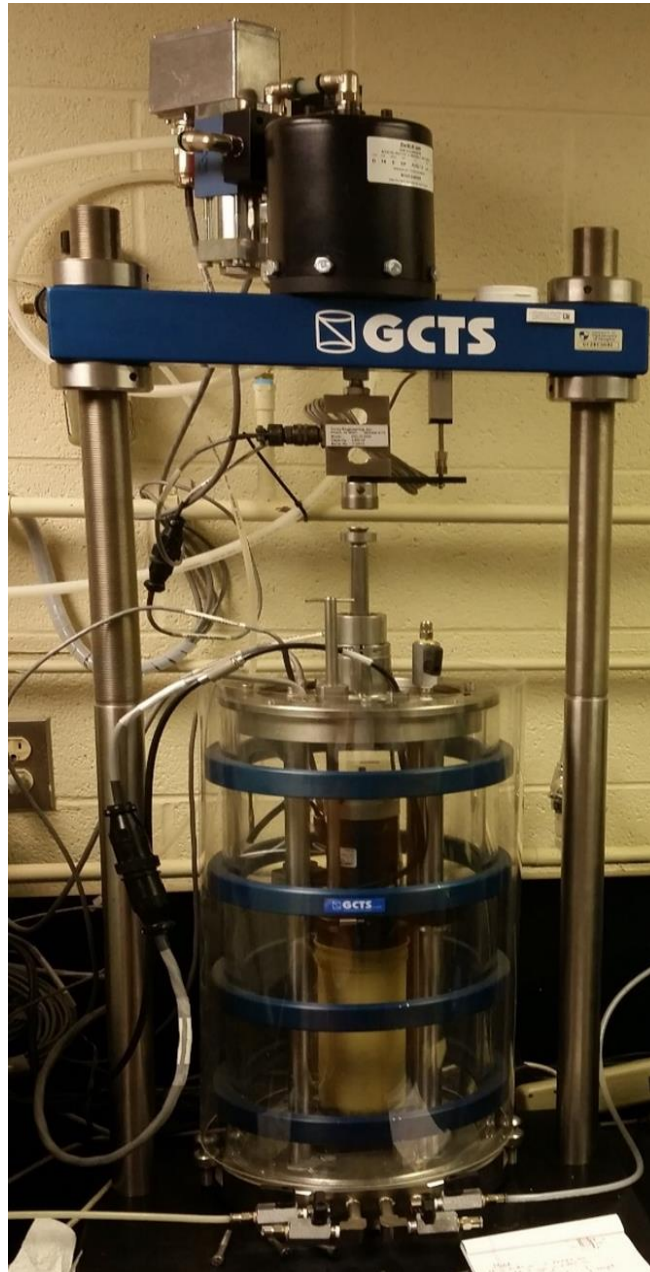
Figure 3.4: Photograph of GCTS Resonant Column & Torsional Shear Equipment
