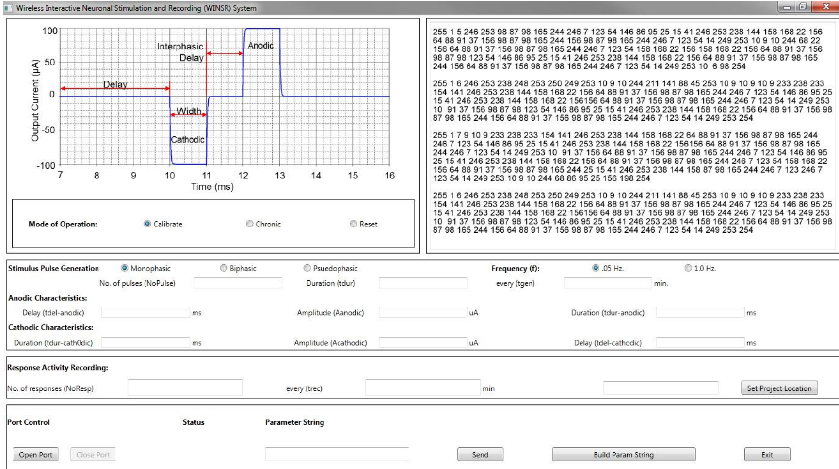
Figure 23 – Screen capture of the Wireless Interactive Neuronal Stimulation and Recording (WINSR) application residing on the host computer (base unit). It is used to interface with the remote unit PCB. Users enter specific experimental controls for stimulus pulse generation and response recording.
