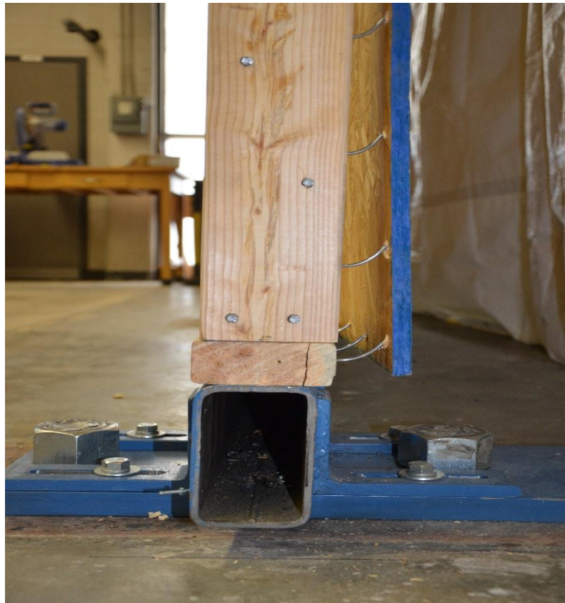
Figure 22. Sheathing failure due to nail slip
