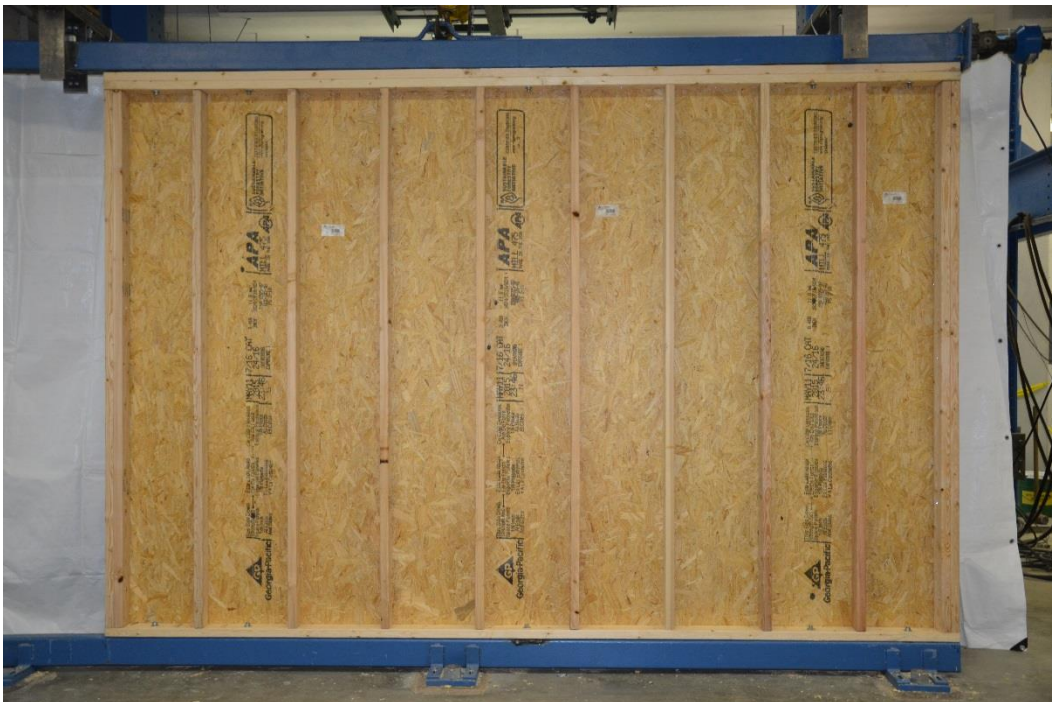
Figure 3. Partially anchored shear wall ready for testing
