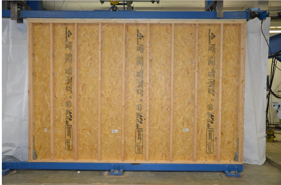
Figure 5. Fully anchored shear wall ready for testing
