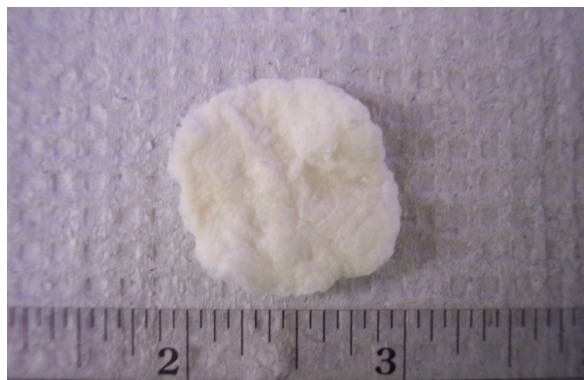
Fig. 1. Photograph of 5 mM DTBP crosslinked chitosan sponge
