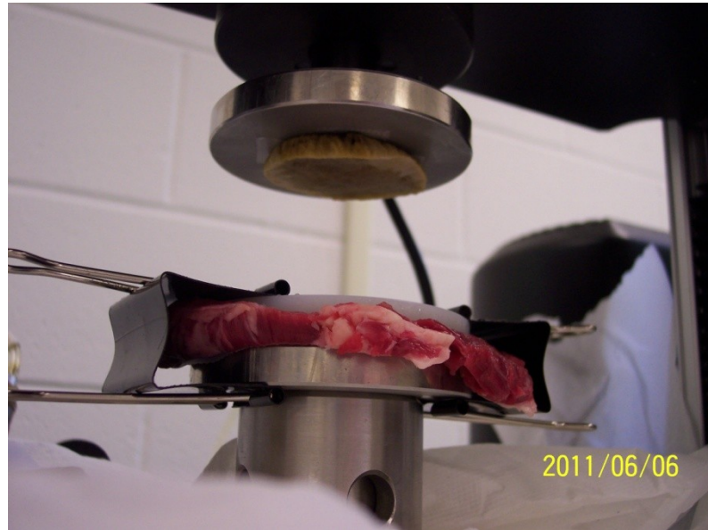
Fig. 4. Bioadhesion testing fixtures with a genipin crosslinked chitosan sponge attached to the top cylindrical fixture of the universal testing machine
