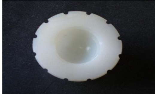
Figure 2: Acetabular cup fabricated from UHMWPE comprises the articulating surface of a total artificial hip.
