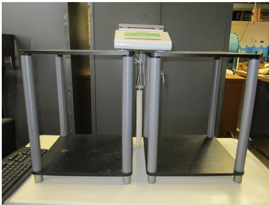
Figure 8. Cylinder hanging vertically underneath scale during procedure.
