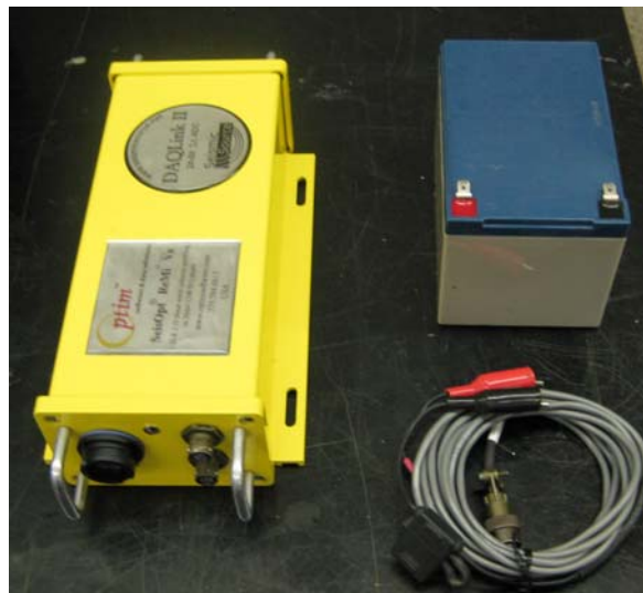
Figure 4.13 DAQLink II with 12-volt battery and power cable.
