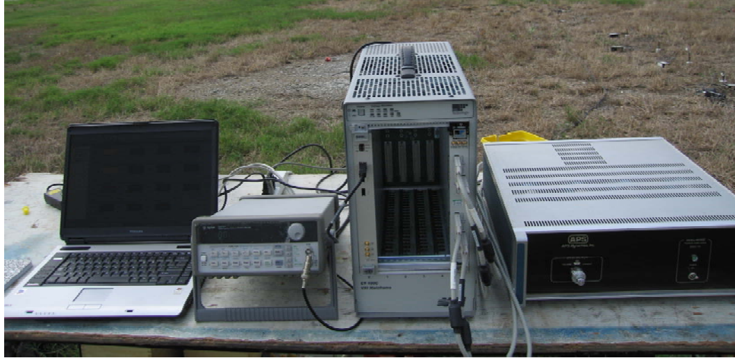
Figure 4.11 Data acquisition Equipment. From left to right: Computer with VEE Pro software; 33120A Function/Arbitrary Waveform Function Generator; CT-100C portable VXIbus mainframe with slotted VT1432A 16-channel 24-bit digitizer; and 144 Dual-Mode Amplifier.
