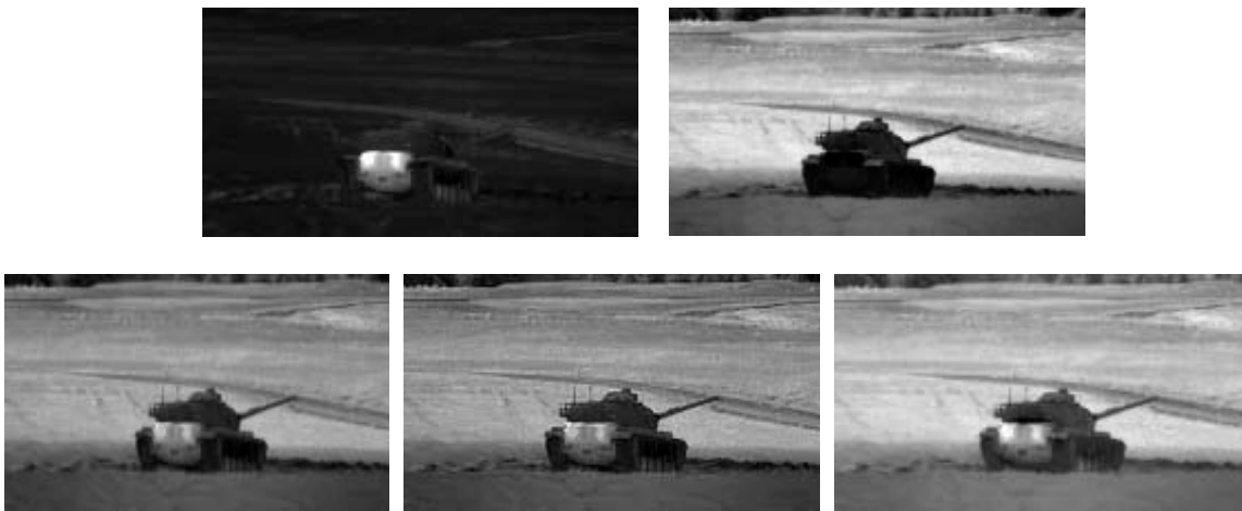
Figure 22. Sample imagery from the LWIR/SWIR 8AFC experiment. Top left is the LWIR image and top right is SWIR image. From left to right, the bottom row shows the superposition, SIDWT and Laplacian fused images.
