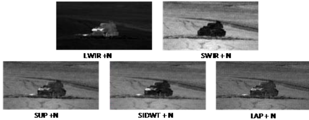
Figure 25a. Fused LWIR and SWIR imagery using three different image fusion algorithms with a SNR of 40 dB imposed on the imagery. SUP-superposition, LAP-Laplacian and SWT- Shift-invariant DWT
