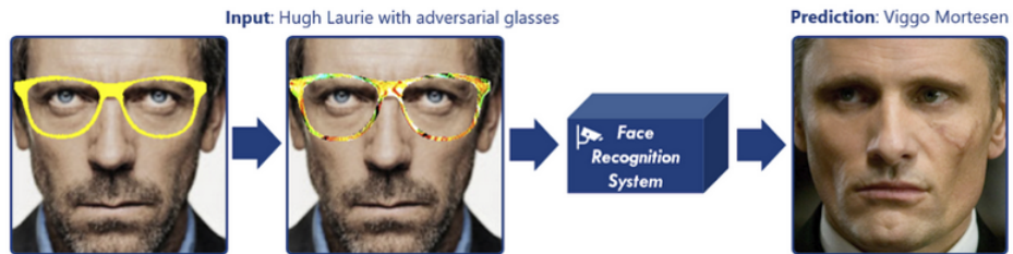
Figure 1.1: Adversarial attack examples on face biometric. Adding a special sunglasses can be able to fool the face biometric.
