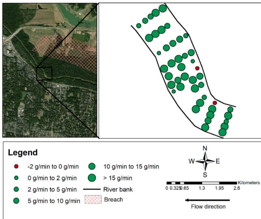
Figure 17. Spatial distribution of seepage rates obtained from installing seepage meters at the finer scale along Sub-reach B, Wolf River.
