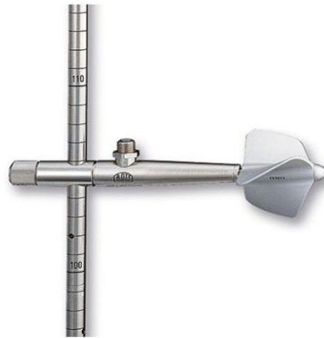
Figure 9. Ott C2 current meter body, rod, and propeller
