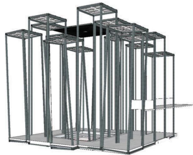
Basic structure of connected container module, which are shifted slightly to allow for slices of light to enter the space
