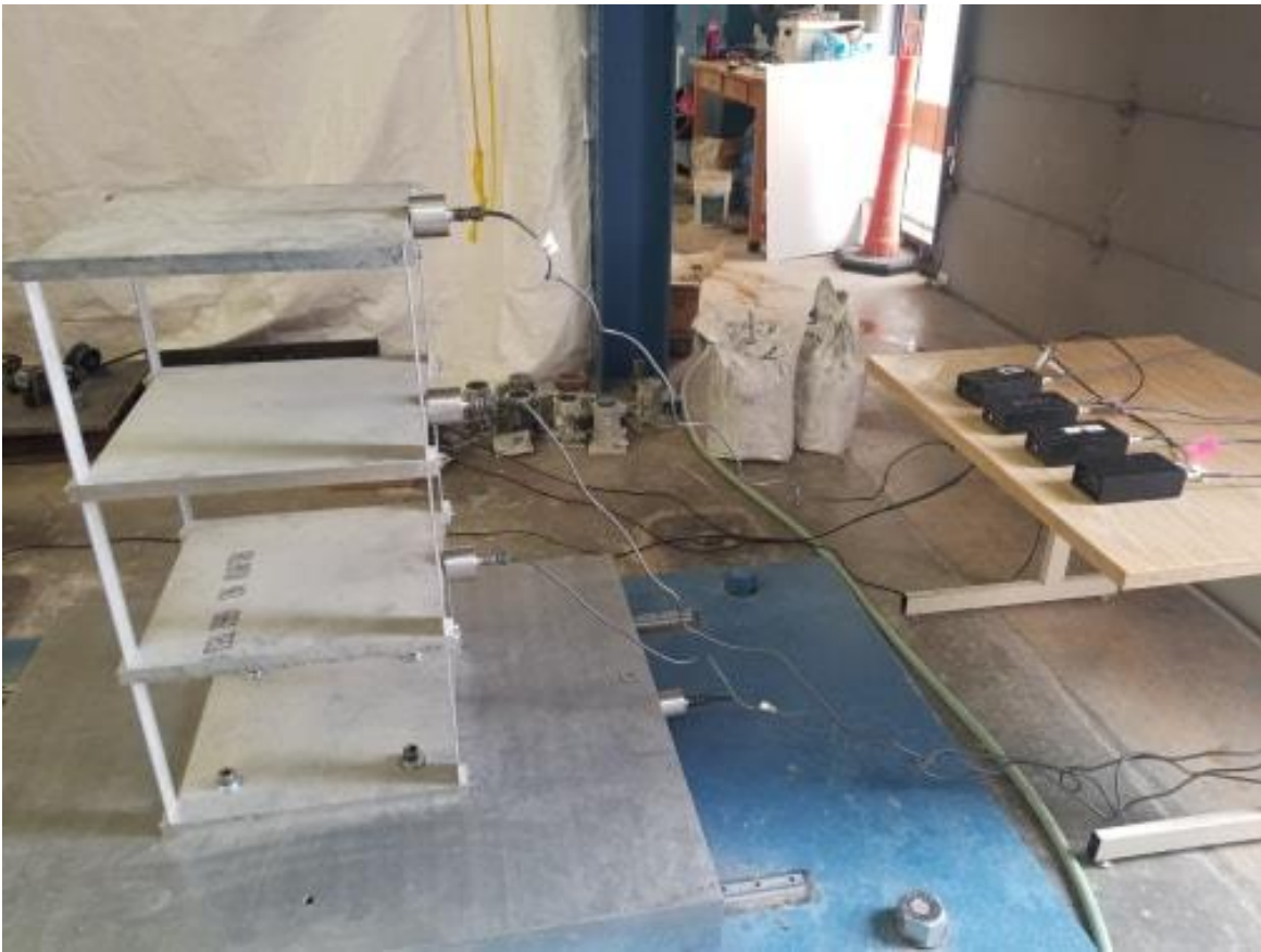
Figure 30. Experimental setup for three-story model
