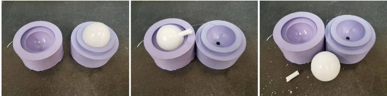
Figure 17: Mold separated, specimen removed, then trimmed fill plug excess, and tied a loop in the string for suspending.
