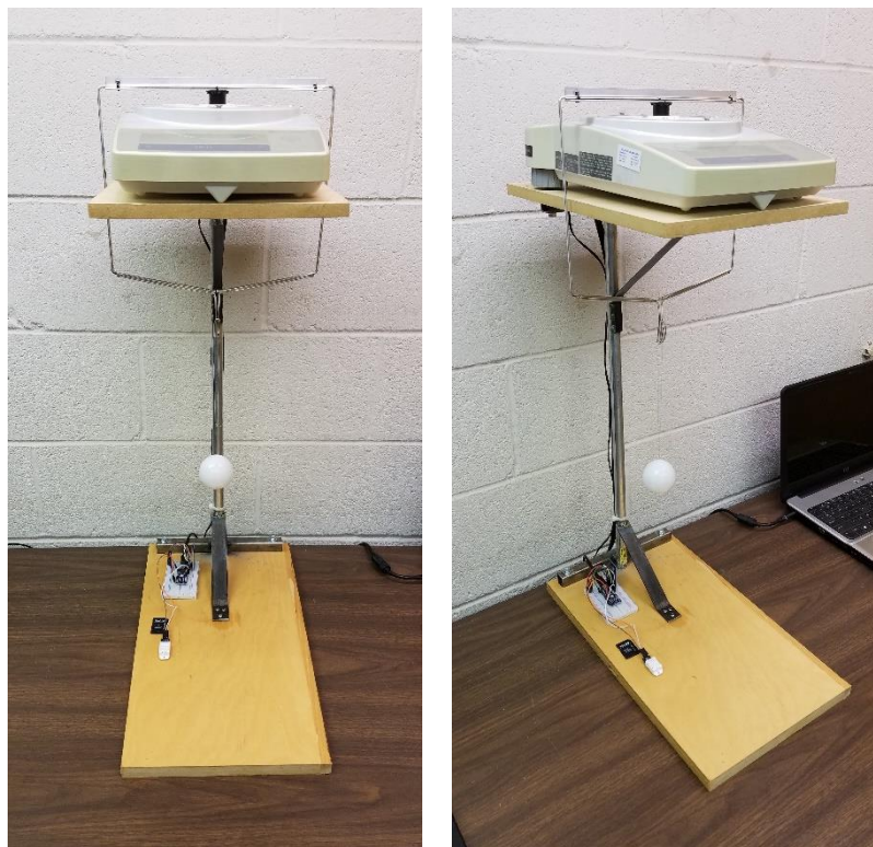
Figure 16: Specimen hung on the weigh below hook and ready for starting mass data acquisition.
