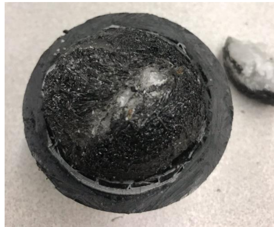
Figure 2: First casting test in ABS mold which was required to be cut open due to the paradichlorobenzene melting the plastic from a chemical reaction.
