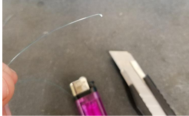
Figure 12: The tip at one end of the fishing line was melted, creating a small ball, to prevent the line from coming out of the cast specimen.
