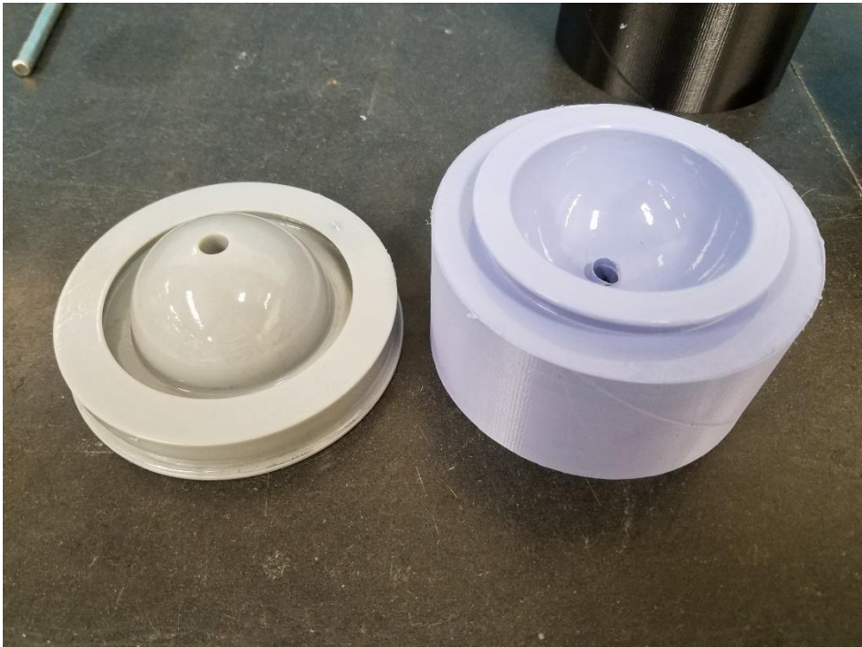
Figure 17: Silicone mold removed from mold negative.
