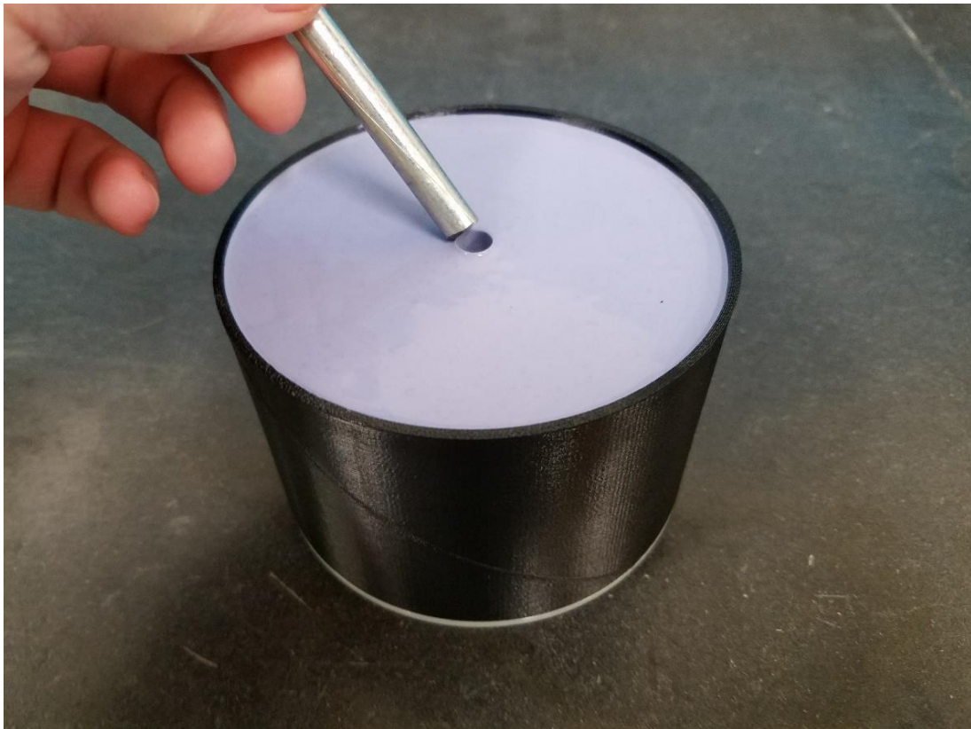
Figure 15: Center post removed, revealing a fill hole.
