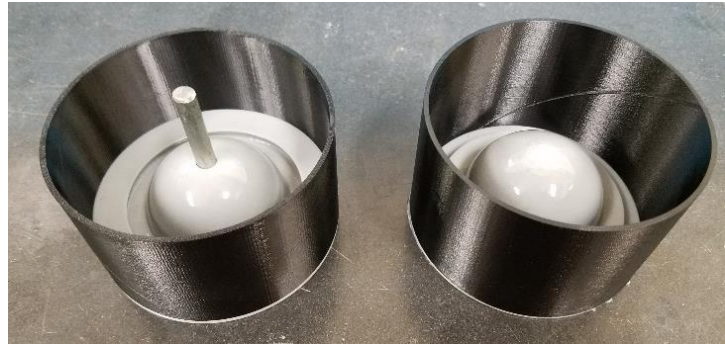
Figure 10: Mold negatives assembled, cleaned and ready to accept silicone.
