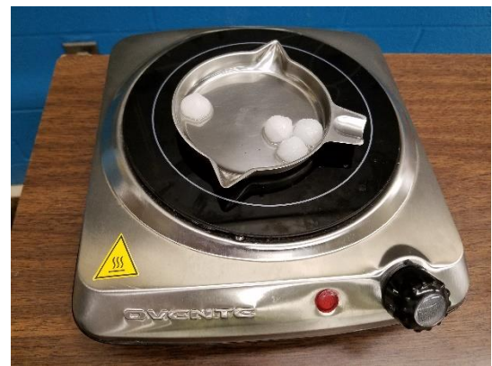
Figure 14: Melting paradichlorobenzene moth balls in stainless-steel dish on electric skillet.
