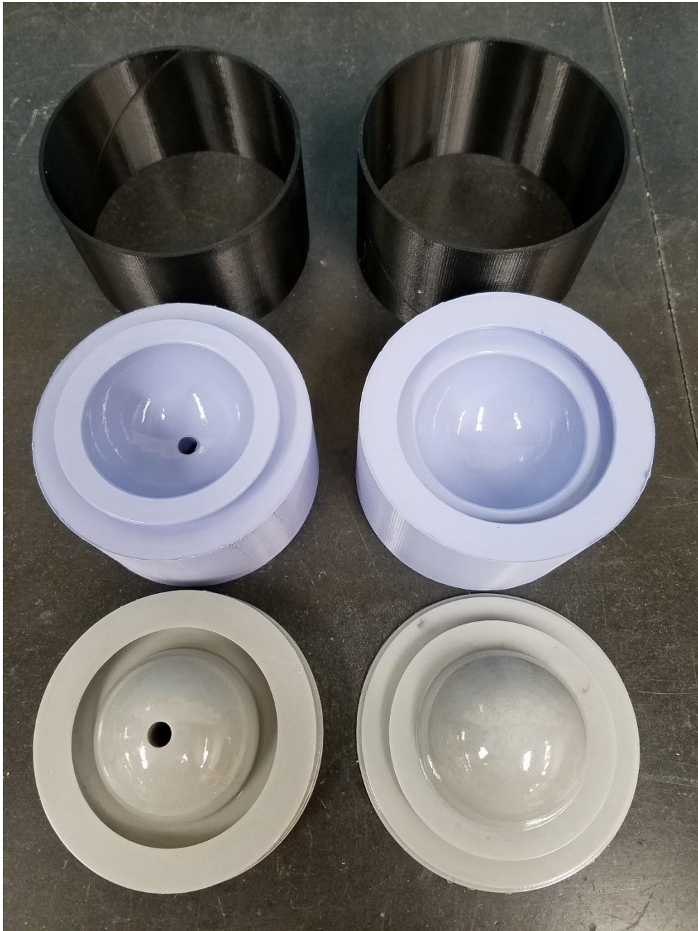
Figure 18: All components disassembled revealing the two silicone mold halves, ready to be used.
