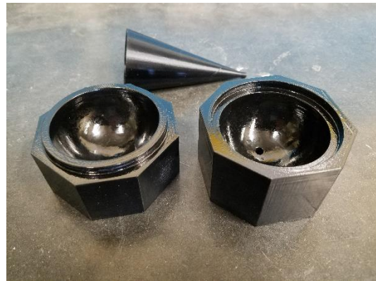
Figure 1: First finished mold made from ABS plastic.
