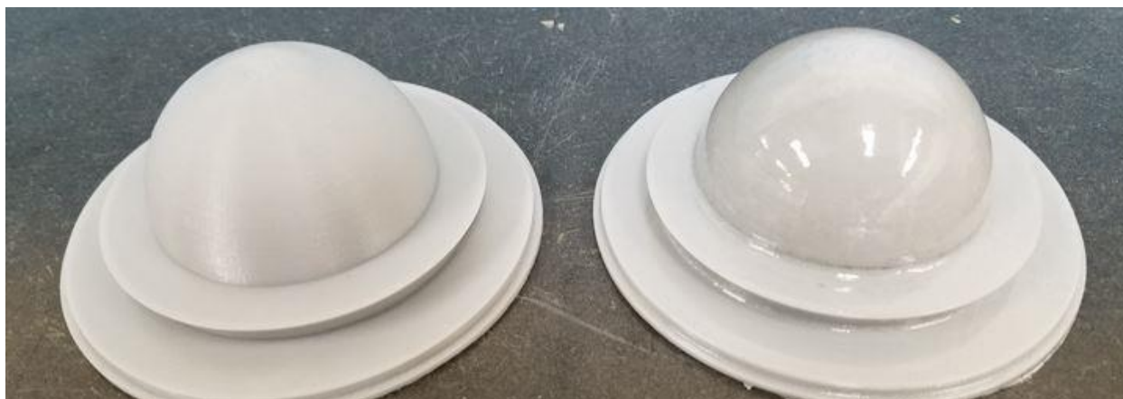
Figure 4: Pictured above, un-altered 3d printed mold negative on the left and acetone vapor smoothed mold negative on the right.
