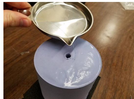
Figure 15: Pouring melted paradichlorobenzene into silicone mold.
