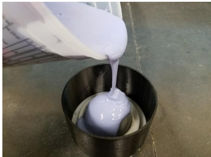
Figure 8: The silicone being poured into mold negatives.
