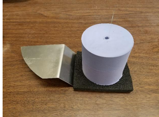
Figure 13: Assembled mold placed on transportation tray with thermal insulation pad.
