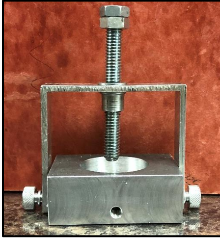
Figure 16: Sample mold and aerogel placement holder.
