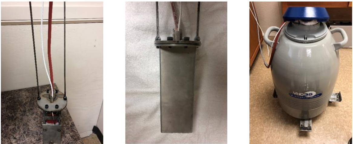
Figure 21. Cryogenic temperature apparatus and measurement setup.
