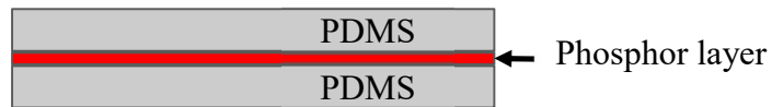
Figure 11: Schematic diagram of PDMS sample made with a layer of phosphor-doped PDMS mirroring Method 2 of the aerogel synthesis configurations used in parallel to the aerogel sample synthesized and used for experimentation via Method 1.
