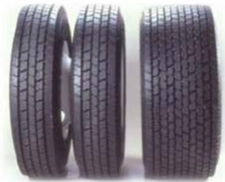
Figure 10. Dual Truck Tire Assembly (Left) and Wide Base Tire Assembly (Right). Adapted from Technologies and Approaches to Reducing the Fuel Consumption of Medium- and Heavy-Duty Vehicles by the Committee to Assess Fuel Economy Technologies for Medium- and Heavy-Duty Vehicles, 2010, p. 112. Copyright 2010 by National Academy of Sciences. Reproduced with permission.
