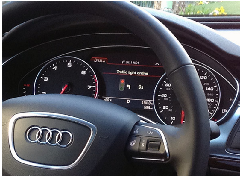
Figure 8. Audi Traffic Light Assist Demonstration. ©2014 by Consumers Union of U.S., Inc. Yonkers, NY 10703-1057, a nonprofit organization. Reprinted with permission from ConsumerReports.org for educational purposes only. No commercial use or reproduction permitted. www.ConsumerReports.org .
