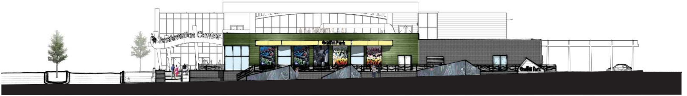
FIGURE 91. West Elevation, by Victor Robinson, 2014. The west elevation displays the public facade of the building. The graffiti zone is located on the pedestal a few feet above the sidewalk to showcase the art to the community. Chalkboard walls are located on the sidewalk level to be easily accessed by the community.
