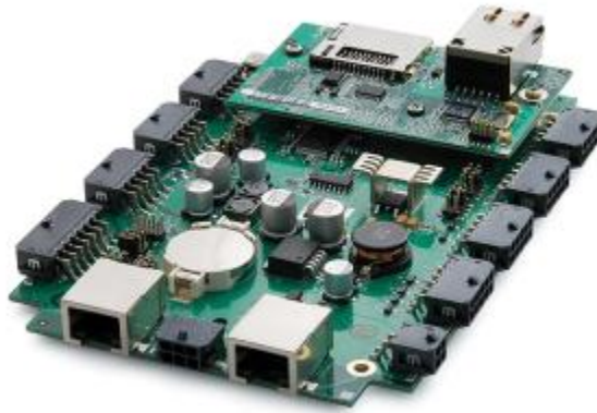
Figure 3-1. Digi® BL4S200 Single Board Computer [17].
