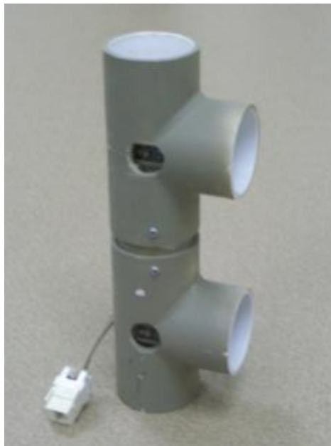
Figure 2-1. Paired detectors mounted within PVC housings.
