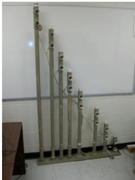
Figure 4-8. Custom profile sensor array prototype realized on PVC pipe.
