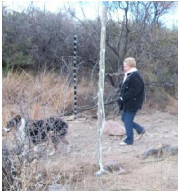
Figure 1-1. Dog and human passing through the parallel detector beams of a sparse sensor array.
