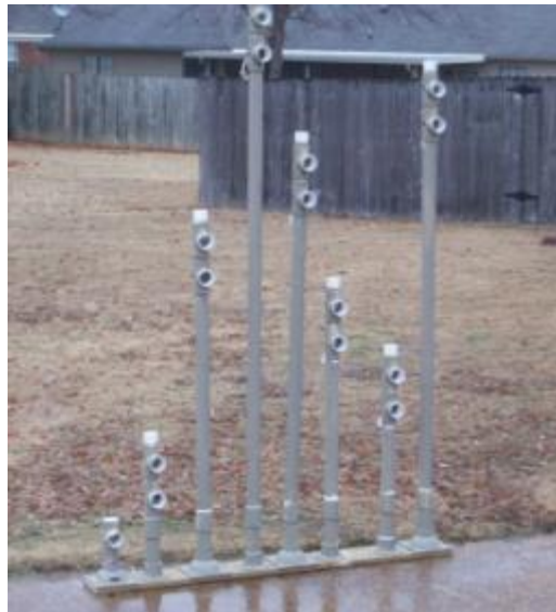
Figure 4-2. Example of custom array implementation using PVC pipe.
