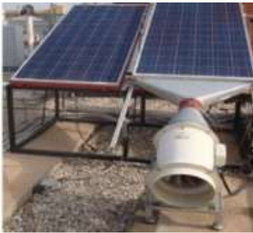
Figure 2. Photovoltaic/Thermal-air system with forced air convection configurations
